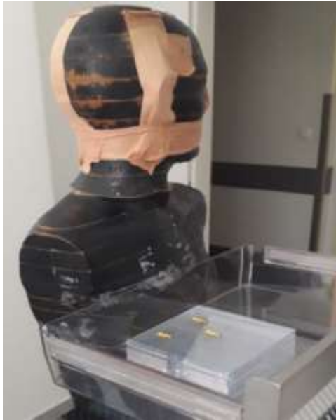
Figure 1- Anthropomorphic phantom and positioning of dosimeters on PMMA plates in the first irradiation plan.
